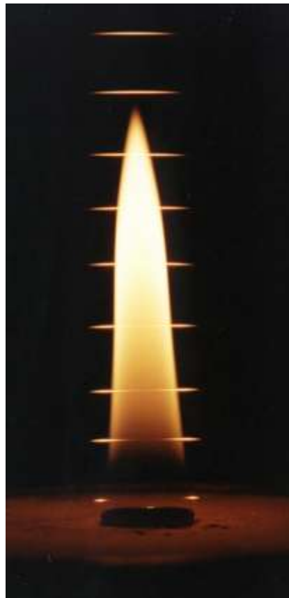
Image of the test flame and glowing Si C fibers. The flame is about 7 cm tall.
