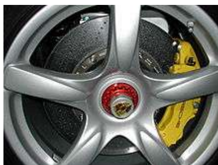
The Porsche Carrera GT's carbon-ceramic (silicon carbide) disc brake
