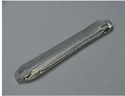
A synthetic silicon dioxide crystal grown by the hydro thermal method, about 19 cm long and weighing about 127 grams
