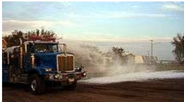
A fire truck demonstrating Class A foam in a CAFS system
