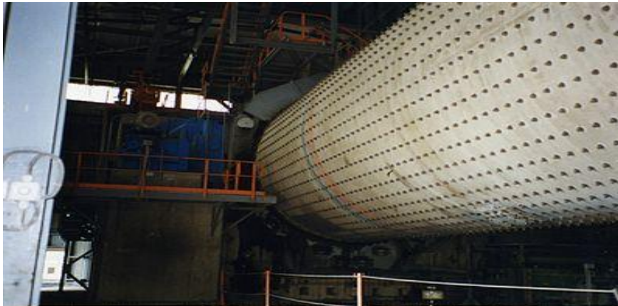
A 10 MW cement mill, output 270 tones per hour
