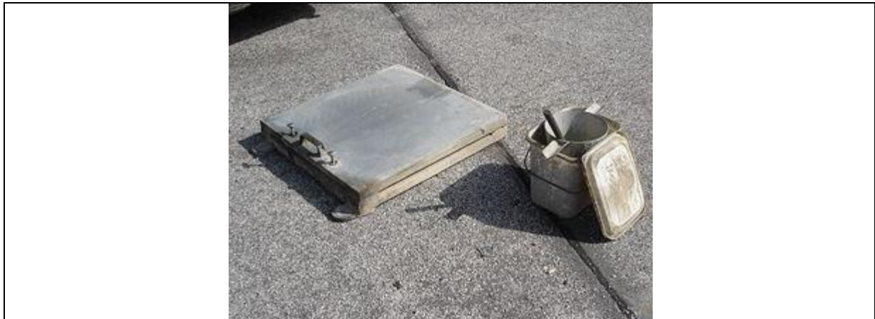
Equipment; flow table, Abrams cone, water bucket and broom.
