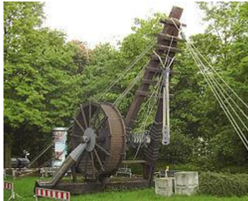
Reconstruction of a 10.4 m high Roman Polyspastos at Bonn , Germany.
