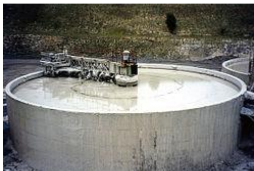
A 1500 m 3 storage tank of slurry, blended and prevented from settling out by a rotating arm injecting compressed air
