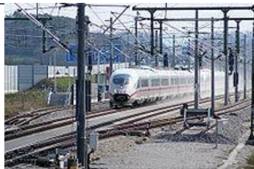
At 300 km / h , an ICE 3 (DB class 403) releases sand from several bogies to the rails.
