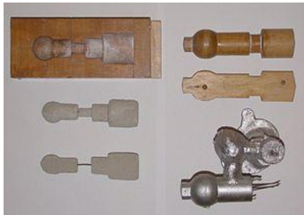
Left : Core box, with resulting (wire reinforced) cores directly below. Right:- Pattern (used with the core) and the resulting casting below (the wires are from the remains of the core)
