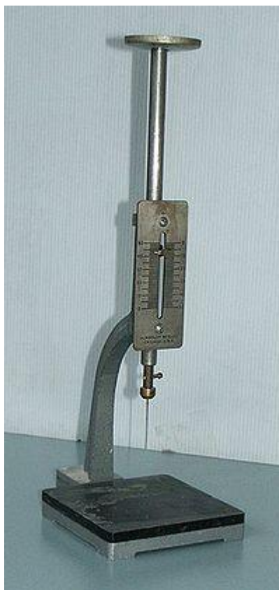
Vicat needle for cement paste solidification time measurement
