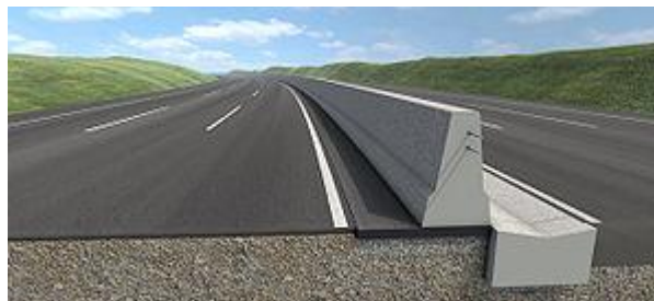
Concrete step barrier cross - section
