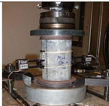
Compression testing of a concrete cylinder
