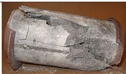
Same cylinder after failure
