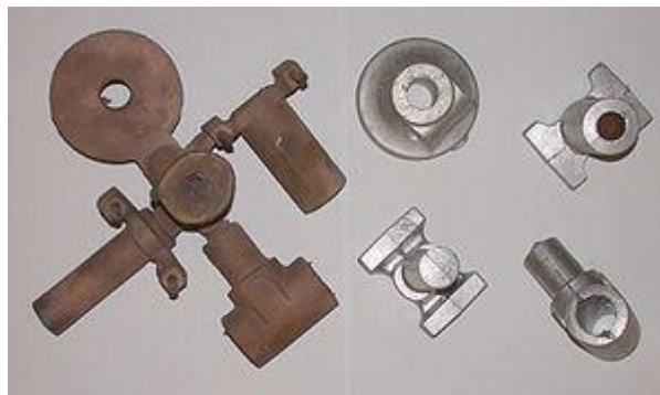
Two sets of castings (bronze and aluminium) from the above sand mold
