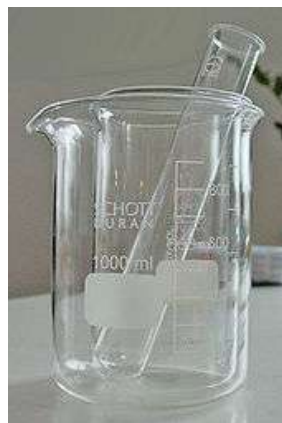
Borosilicate glassware. Displayed are two beakers and a test tube.
