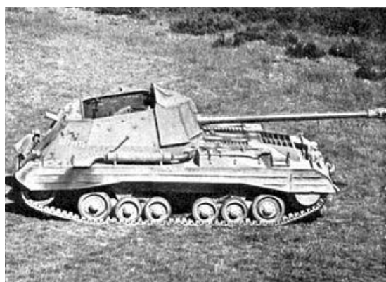
A British Archer tank destroyer, based on the hull of a Valentine tank
