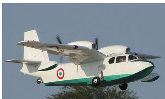
Italian Air Force Piaggio P.136 during takeoff retracting the wheels that make it an amphibian.
