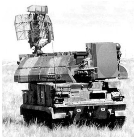
The Russian Tor missile system can engage targets while moving, thus achieving high survivability.
