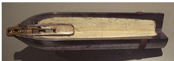
Picric acid was used in the first high explosive shells. Cut out section of a high explosive shell belonging to a Canon de 75 modèle 1897.
