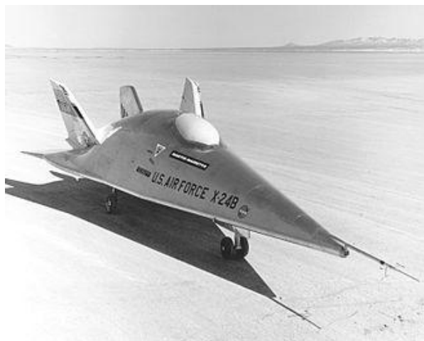
X-24B lifting body, specialized glider
