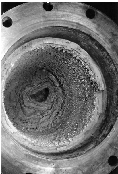
After the reaction, remnant slag coats the interior of a bomb.
