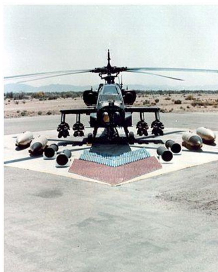
Weapon loadout of the AH-64 Apache Data from Jane's Information Group, Bishop
