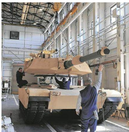
Mechanics at Anniston Army Depot line up an M1 Abrams turret with its hull.
