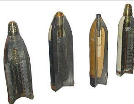
Some sectioned shells from the First World War. From left to right: 90 mm fragmentation shell, 120 mm pig iron incendiary shell, 77/14 model - 75 mm high explosive shell, model 16-75 mm fragmentation shell
