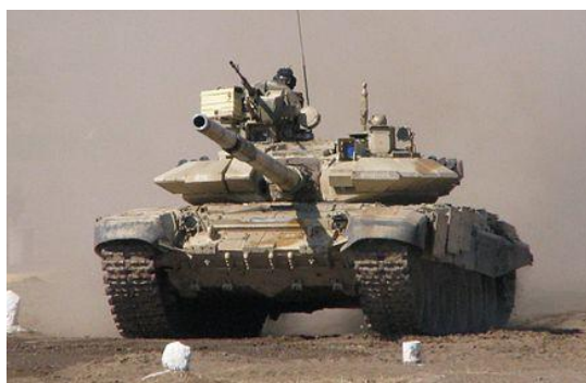
Indian T-90 Bhishma with appliqué reactive armor and standard 125 mm main gun
