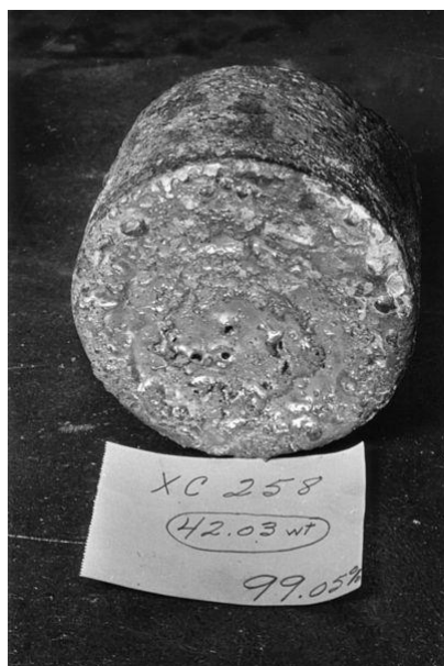
A uranium metal "biscuit" from the reduction reaction
