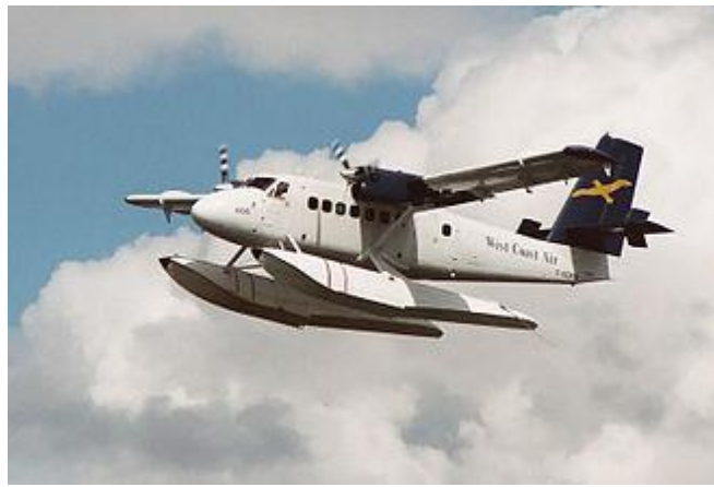
A turboprop- engined DeHavilland Twin Otter adapted as a floatplane
