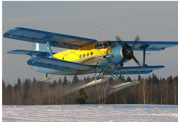
An-2R on skis allowing operations in the snow
