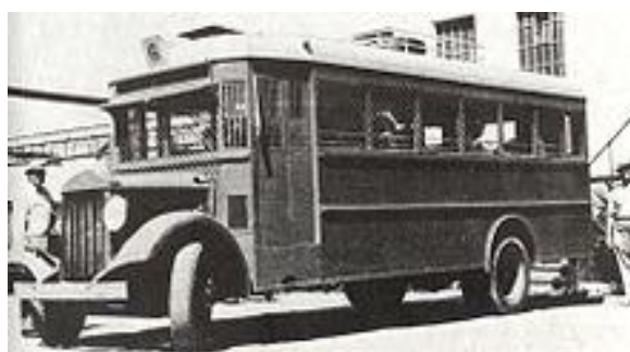
A Jewish bus equipped with wire screens to protect against rock, glass, and grenade throwing, late 1930s
