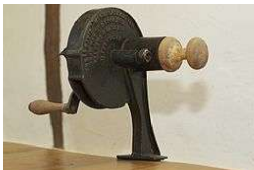
Antique marmalade cutter, a device used to cut the peel of the citrus fruit into thin slices for the marmalade
