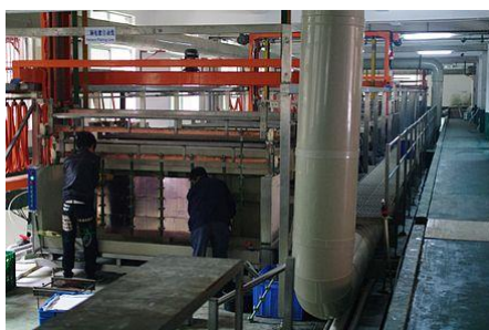
Copper electro plating machine for layering PCBs
