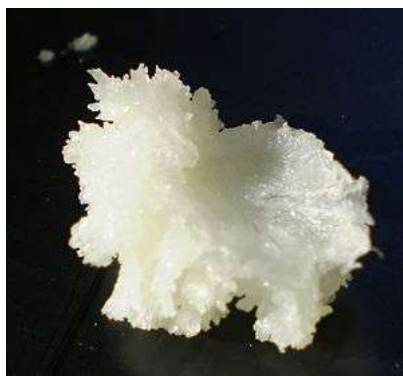
Methyl cinnamate crystals extracted using steam distillation from Eucalyptus olida .
