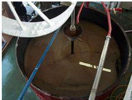
A mash tun full of grain steeping in heated "liquor" (water)
